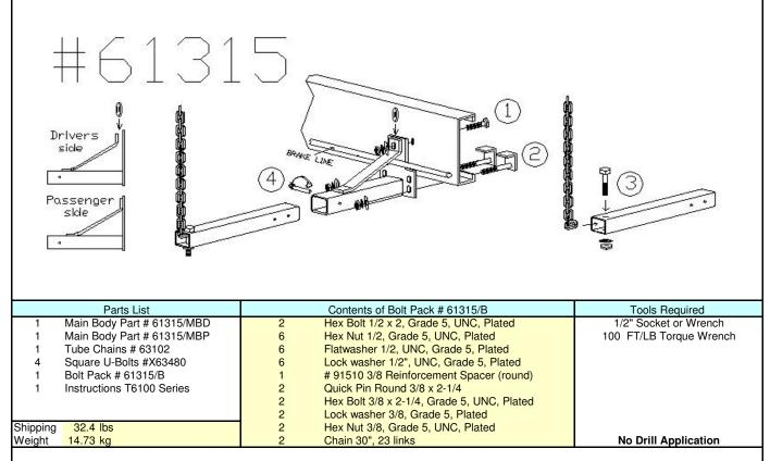
1) Start with the driver's side installation. The driver's side main body has a gap to slide the brake cable through (not applicable to all truck models). Locate hole (1) in side of frame. Place 1/2" x 2" hex bolt through frame and main body with the 3/8 spacer and secure in place loosely with flatwasher, lock washer and nut (as shown in diagram).
