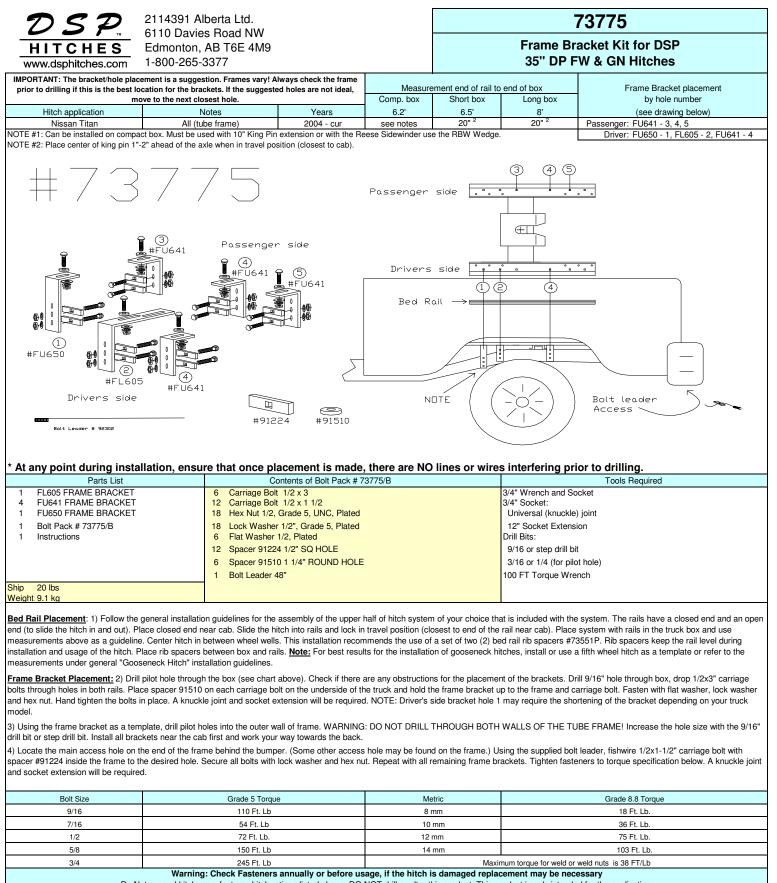
Do Not exceed hitch manufactures hitch ratings listed above, DO NOT drill or alter this product. This product is only intended for the application listed above, see vehicle owner's manual for maximum towing capacity (GVWR). This product is intended for usage with the correct towing
